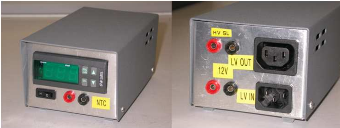
Figure 12: Temperature interlock schematic and pictures of the unit. The input signal was the resistance read from one NTC on the hybrid. The current temperature was shown in the front panel display. The unit used two relays to interlock both high voltage and low voltage units. On the back panel the HV safety loop and Agilent power cable were connected. If a module overheats both connections are opened and the module power supplies are turned off.
