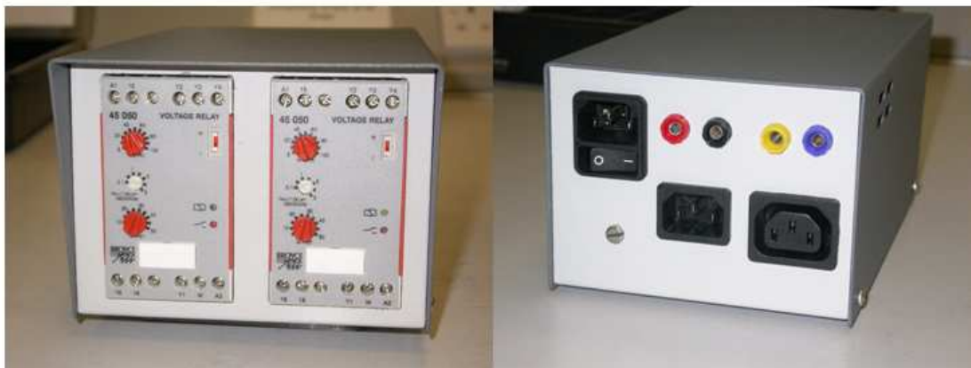
Figure 13: The top picture shows the pressure interlock schematic. The input signal was the 0-5 V delivered by the Controller 201 unit in the vacuum pump system. It used two relays to interlock both high voltage and low voltage units. The state of the relays can be verified from the LEDs on the front panel. The overvoltage and hysteresis are tuned on the front panel buttons. On the back panel the HV safety loop and Agilent power cable are connected.
