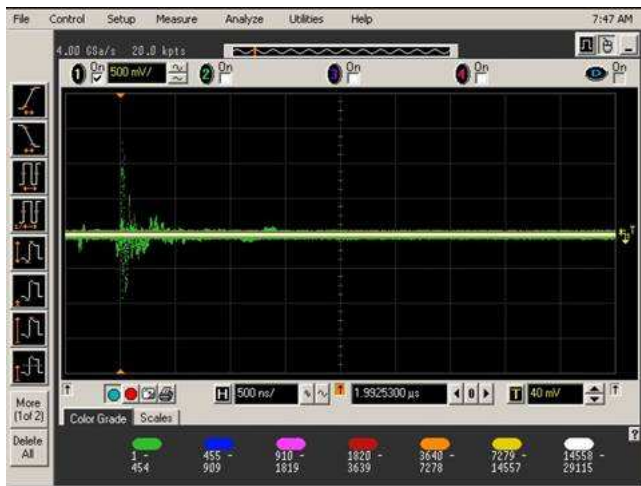
Figure 12: Oscilloscope trace of the output voltage during a brown-out when it is in persistency mode. The voltage scale is 500mV/division. The time scale is 500ns/division.
