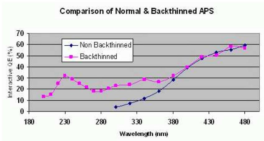
Figure 3: Measurement of the interactive QE for the normal and backthinned Vanilla APS
