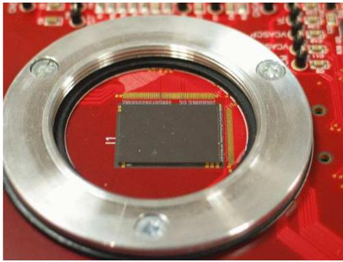
Figure 2: Picture of the BT Vanilla sensor bonded to PCB
