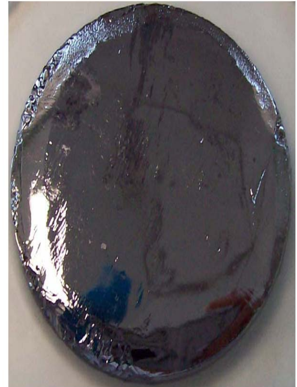
M4_019, 50 mm diameter CZT boule grown in new MTPVT system
